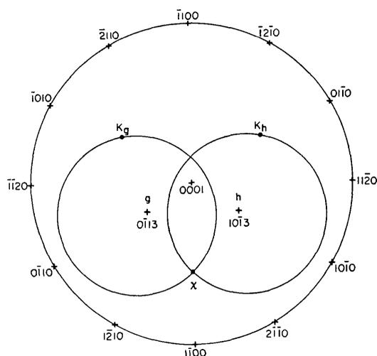
Fig. 1. Stereographic (0001) projection for zinc showing reflection loci for  $\text{Co } K\alpha$  from  $0\bar{1}13$  and  $10\bar{1}3$  planes with poles  $g$  and  $h$ . With incident beam  $\chi$ , the two reflected beams  $K_g$  and  $K_h$  have an  $84^\circ$  stereo separation angle. The scratch direction was  $[1\bar{1}00]$  which produced dislocations with a  $\frac{1}{3}[11\bar{2}0]$  Burgers vector.
